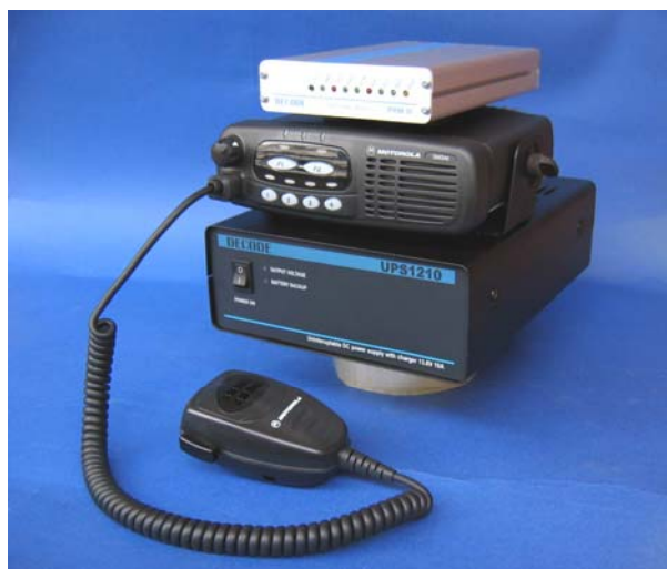
Uninterruptible power supply UPS 1210a in use with radio station and with DECODE packet radio modem PRM III
